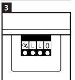
The terminal block is now accessible. In the right L and in the 0 come the supply wires. Connect the brown wire to the right L and the blue wire to the 0. On the left side, we connect the descending side. Then connect the black wire to the switch sign (left side). And the brown wire to the left L.
