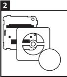
Remove the rotary/pushbutton from the dimmer by pulling it. Then loosen the nut, and remove the rosette from the dimmer.
