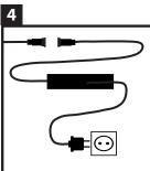
Now connect the LED ground light to the Hamulight (Astro) LED transformer through the simple screw system. Finally, insert the plug of the transformer into a
