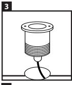
Drill the holes, size 43 mm, at the desired place. The LED ground light must be placed through the hole in the tube before it is connected to the power.
