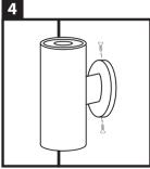
Mount the wall light on the base with the 2 screws.
