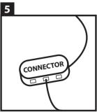
Now connect the LED wall light to the connector of the LED veranda set. Note: you must have a free port in your connector.
