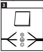
Now you can connect the LED wall light to an on/off switch. N = blue wire, L = brown wire and = = yellow/green wire. We recommend to switch off the branch circuit beforehand!
