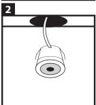
Drill the holes, size 28 mm, at the desired place. Next, position the wiring of the LED spots on the desired location. Place the LED spots in the drill holes. Bring the recessed spotlight into place, the spotlight snaps into place with the spirals.
