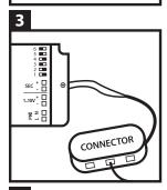
Subsequently, link all the spots to the connector. The plugs should all be linked to the connector, as the system is connected in series. If the connector contains more ports than the amount of installed spots, please place a jumper (black jumper) in the remaining opening(s). Jumpers will be provided in the box (depending on the amount of spots and the type of connector).
