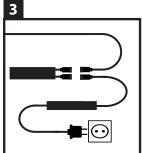
Now connect the LED strip to the wifi veranda LED receiver. You do this by connecting the couplers. Do you have several LED strips? Then you need to connect the LED strips to the cable connector that you connected to the wifi veranda LED receiver before.
