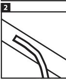
Place the LED strip in the desired location. Remove the 3M tape from the LED strip and then paste it into the profile.
