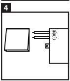
Now you can connect the transformer to an an on/off switch. PRI N =blue wire and PRI L =brown wire. We recommend to switch off the branch circuit beforehand!
