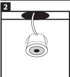
Drill the holes, size 35 mm, at the desired place. Next, position the transformer of the LED spots on the desired location. Place the LED spots in the drill holes. Now you can push the two spirals against the spot to move it into position.
