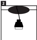
Drill the holes, size 80 mm, at the desired place. Now you can connect the fitting (through the hole) to an electric current. We recommend to switch off the branch circuit beforehand!
