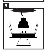
Now you can push up the two spirals and move the spot into position. Next, connect the LED spots to the fitting. Then position the LED recessed spot in the fixture. The inner ring must be removed. Your lightening is now ready for use.
