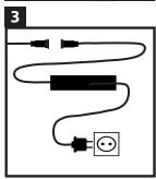
Now connect the LED strip to your 24-volt Hamulight transformer. Plug the transformer into a socket.
