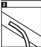
Place the LED strip in the desired location. Remove the 3M tape from the LED strip and then paste it into the profile.
