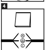
Now you can connect the LED ground light to power. N = blue wire, L = brown wire and  $\implies = yellow/green$  wire. We recommend to switch off the branch circuit beforehand!
