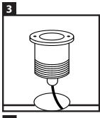
Drill the holes, size 43 mm, at the desired place. The LED ground light must be placed through the hole in the tube before it is connected to the power. We recommend handling the cable at least 50cm below ground level.
