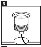
Drill the holes, size 85 mm, at the desired place. The LED ground light must be placed through the hole in the tube before it is connected to the power. We recommend handling the cable at least 50cm below ground level.
