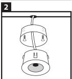
Drill the holes in the desired position in your veranda. First position the cables of the LED surface-mounted spotlight at the desired location. Attach the cables to the drill hole and screw the recess into the profile and click the LED surface-mounted spotlight into the recess.
