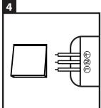
Now you can connect the transformer to a 230V point (INPUT). ←= green/yellow wire, N = blue wire and L = brown wire. We recommend to switch off the branch circuit beforehand! If you are connecting the spots to the main current, please link the transformer's INPUT with an on/off switch of the main current.
