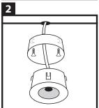
Drill the holes at the desired place on your veranda. Next, position the wiring of the LED spots on the desired location. Place the wiring in the drill hole and screw the armature in the profile. Click the mounted spot in the armature.
