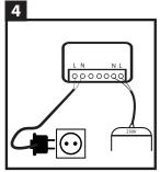
Now you can connect the Wifi LED receiver to the transformer. N = blue wire and L = brown wire. We recommend to switch off the branch circuit beforehand! If you are connecting the spots to the main current, please link the transformer's INPUT with an on/off switch of the main current.
