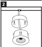
Drill the holes at the desired place on your veranda. Next, position the wiring of the LED surface-mounted spotlights on the desired location. Place the wiring in the drill hole and screw the armature in the profile. Click the mounted spot in the armature.
