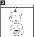
Drill the holes at the desired place on your veranda. Next, position the wiring of the LED spots on the desired locatioein. Place the wiring in the drill hole and screw the armature in the profile. Click the mounted spot in the armaturce.
