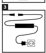
Now connect the standing light with the simple screw system and the Hamulight (astro) LED transformer. Finally, connect the plug of the transformer into a socket.
