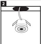
Drill the holes, size 53 mm, at the desired place. Next, position the transformer of the LED spots on the desired location. Place the LED spots in the drill holes. Now you can push up the two spirals and move the spot into position.
