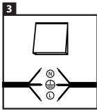
Now you can connect the LED ground spot to power. N = blue wire, L = brown wire and  $\bigoplus = yellow/green$  wire. We recommend to switch off the branch circuit beforehand!
