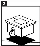
Make a 90 x 90 mm hole at the desired place. Place the LED ground light in the hole. We recommend handling the cable at least 50cm below ground level.
