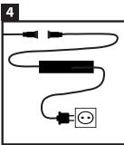
Now connect the LED spike light to the Hamulight (Astro) LED transformer through the simple screw system. Finally, insert the plug of the transformer into a socket.
