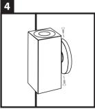
Mount the wall light on the base with the 2 screws
