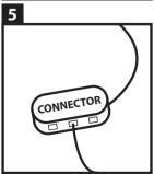
Now connect the LED wall light to the connector of the LED veranda set. Note: you must have a free port in your connector.
