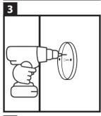
Secure the base to the wall with two screws at the desired location.
