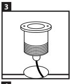
Drill the holes, size 70 mm, at the desired place. The LED ground light must be placed through the hole in the tube before it is connected to the power.
