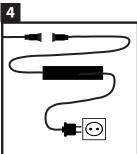
Now connect the LED ground light to the Hamulight (Astro) LED transformer through the simple screw system. Finally, insert the plug of the transformer into a socket.
