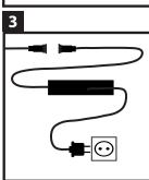
Now connect the standing light with the simple screw system and the Hamulight (astro) LED transformer. Finally, connect the plug of the transformer into a socket.
