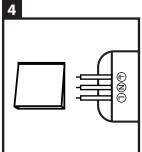
Now you can connect the transformer to a 230V point (INPUT).  $\leftarrow$  green/yellow wire, N = blue wire and L = brown wire. We recommend to switch off the branch circuit beforehand! If you are connecting the spots to the main current, please link the transformer's INPUT with an on/off switch of the main current.
