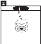
Drill the holes, size 22 mm, at the desired place. Next, position the wiring of the LED spots on the desired location. Place the LED spots in the drill holes. Bring the recessed spotlight into place, the spotlight snaps into place with the spirals.
