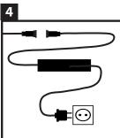
Now connect the LED ground light to the Hamulight (Astro) LED transformer through the simple screw system. Finally, insert the plug of the transformer into a socket
