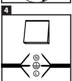
Now you can connect the LED ground light to power. N = blue wire, L = brown wire and  $\implies = yellow/green$  wire. We recommend to switch off the branch circuit beforehand!
