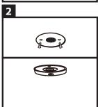
Attach the bracket to the desired position using two screws.
