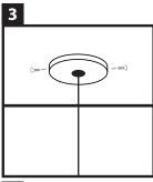
Attach the pendant lamp to the base using the 2 screws.
