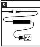
Now connect the wall light with the simple screw system and the Hamulight (astro) LED transformer. Finally, connect the plug of the transformer into a socket.
