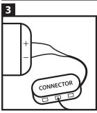
Subsequently, link all the spots to the connector. Not all ports need to be filled, as the system is connected in parallel. It does not matter if the connector contains more ports than the number of spots installed. You can leave these ports open.
