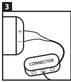
Subsequently, link all the spots to the connector. The plugs should all be linked to the connector, as the system is connected in series. If the connector contains more ports than the amount of installed spots, please place a jumper (black jumper) in the remaining opening(s). Jumpers will be provided in the box (depending on the amount of spots and the type of connector).
