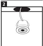
Drill the holes, size 30 mm, at the desired place. Next, position the wiring of the LED spots on the desired location. Place the LED spots in the drill holes. Bring the recessed spotlight into place, the spotlight snaps into place with the spirals.
