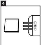
Now you can connect the transformer to a 230V point (INPUT).  $\leftarrow$  green/yellow wire, N = blue wire and L = brown wire. We recommend to switch off the branch circuit beforehand! If you are connecting the spots to the main current, please link the transformer's INPUT with an on/off switch of the main current.
