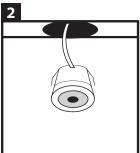
Drill the holes, size 30 mm, at the desired place. Next, position the wiring of the LED spots on the desired location. Place the LED spots in the drill holes. Bring the recessed spotlight into place, the spotlight snaps into place with the spirals.
