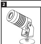
Mount the spike to the spot with the supplied screws.
