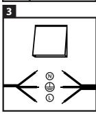
Now you can connect the LED wall light to an on/off switch. N = blue wire, L = brown wire and = = yellow/green wire. We recommend to switch off the branch circuit beforehand!
