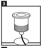
Drill the holes, size 70 mm, at the desired place. The LED ground light must be placed through the hole in the tube before it is connected to the power. We recommend handling the cable at least 50cm below ground level.
