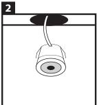
Drill the holes, size 35 mm, at the desired place. Next, position the wiring of the LED spots on the desired location. Place the LED spots in the drill holes. Bring the recessed spotlight into place, the spotlight snaps into place with the spirals.
