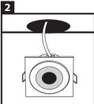
Drill the holes, size 42 mm, at the desired place. Next, position the transformer of the LED spots on the desired location. Place the LED spots in the drill holes. Now you can push up the two spirals and move the spot into position.
