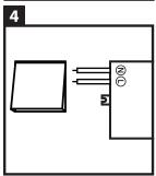
Now you can connect the transformer to an an on/off switch. PRI N =blue wire and PRI L =brown wire. We recommend to switch off the branch circuit beforehand!
