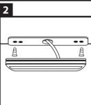
Attach the bottom of the Tarifa surface-mounted spotlight to the beam with the 2 screws. Drill a hole in the middle for the cable to pass through. Place the top of the Tarifa spotlight on the mounted underside. This is magnetic so the spotlight will stay on this way.
