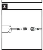
Attach the cable of the Tarifa spotlight to the cable of the 24-volt veranda transformer. Should you use extension cables and/or cable connectors, you will need to connect the spotlight to these. The other cable can be used to connect to another spotlight.
