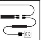
Now connect the Tarifa spotlight to the 24 volt Somfy io veranda LED receiver. You do this by connecting the couplers. Do you have several Tarifa spotlights? Then you need to connect the spots to the cable connector that you connected to the Somfy io veranda LED receiver before.
