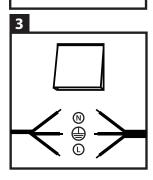
Now you can connect the LED standing light to an on/off switch. N = blue wire, L = brown wire and = yellow/green wire. We recommend to switch off the branch circuit beforehand!
