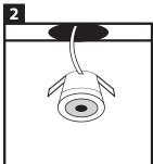
Drill the holes, size 42 mm, at the desired place. Next, position the wiring of the LED spots on the desired location. Place the LED spots in the drill holes. Now push up both spirals and position the spotlight.
