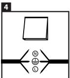
Now you can connect the LED ground light to power. N = blue wire, L = brown wire and = yellow/green wire. We recommend to switch off the branch circuit beforehand!
