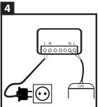
Now you can connect the Wifi LED receiver to the transformer. N = blue wire and L = brown wire. We recommend to switch off the branch circuit beforehand! If you are connecting the spots to the main current, please link the transformer's INPUT with an on/off switch of the main current.
