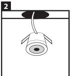
Drill the holes, size 30 mm, at the desired place. Next, position the wiring of the LED spots on the desired location. Place the LED spots in the drill holes. Now push up both spirals and position the spotlight.
