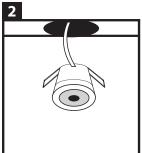
Drill the holes, size 30 mm, at the desired place. Next, position the wiring of the LED spots on the desired location. Place the LED spots in the drill holes. Now push up both spirals and position the spotlight.
