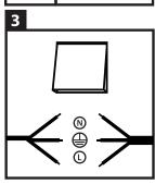
Now you can connect the LED wall light to an on/off switch. N = blue wire, L = brown wire and  $\bigoplus = yellow/green$  wire. We recommend to switch off the branch circuit beforehand!
